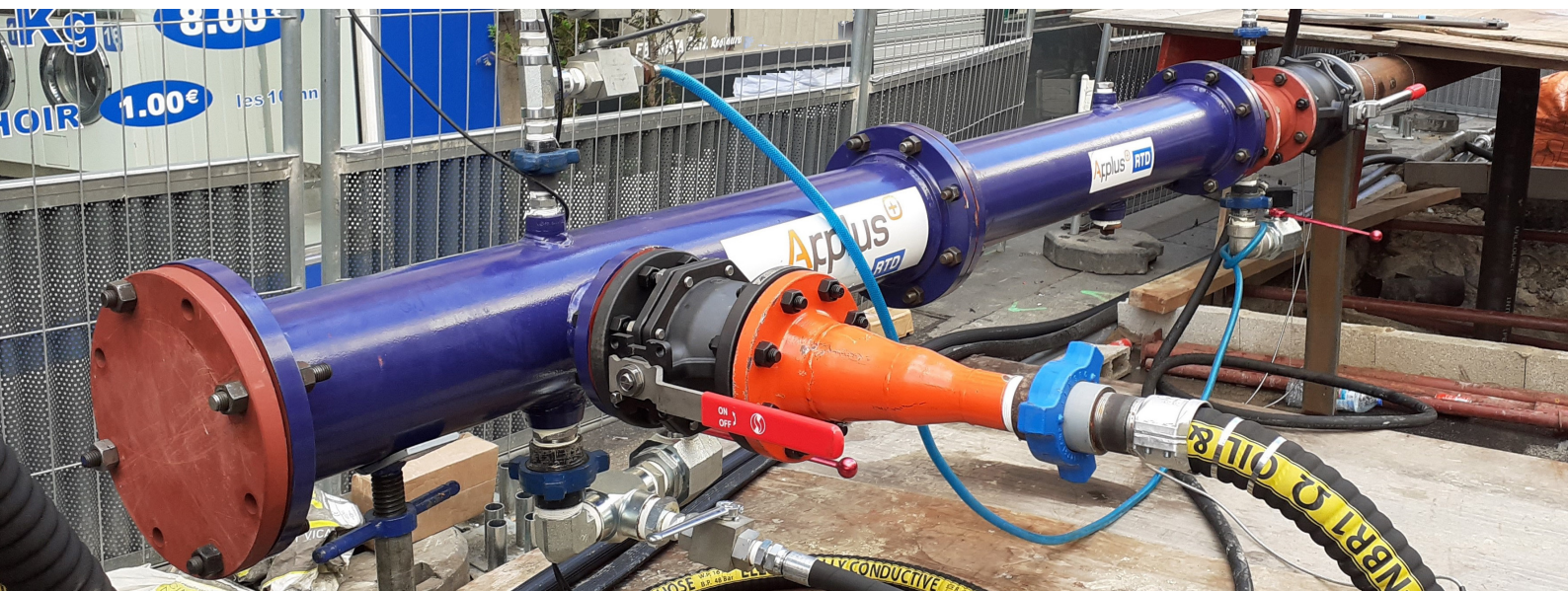
Temporary Launcher facility
