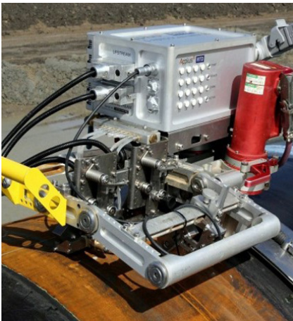
New Construction weld inspection
